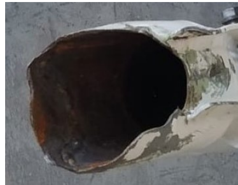
Photograph 9. Corrosion on fragment 3
