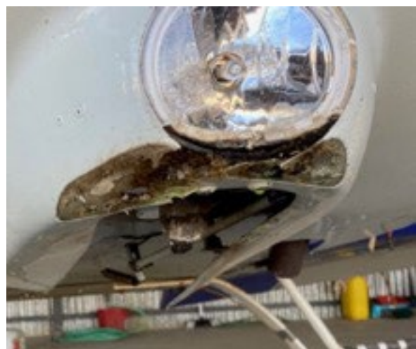
Photograph 5. Nose landing gear housing damage
