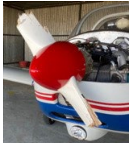
Photograph 6. Damage to the propeller
