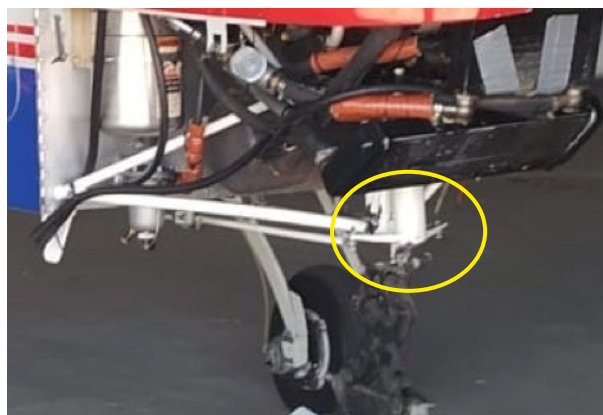
Photograph 10. Assembly accessory for attaching the nose gear leg to the engine mount
