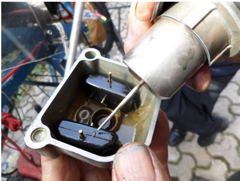
Fig. 6: Metallic impurities in the float bowl of the carburetor for cylinders 2 and 4
