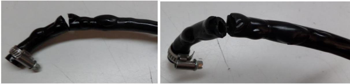
Fig. 5: Fuel hoses in poor condition
