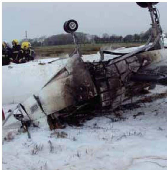
Photo No. 10: Right Engine Fire damage
