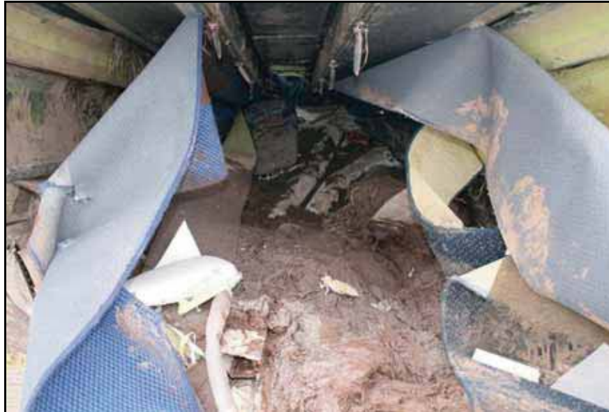
Photo No. 11: Forward view of inverted passenger cabin following rescue operation
