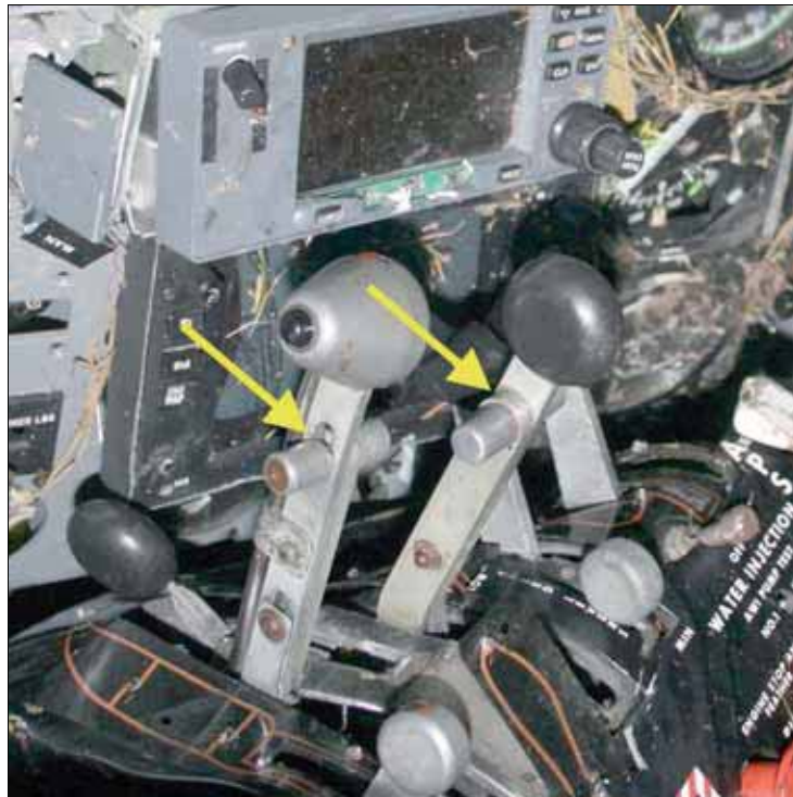
Photo No. 8: Left and Right Beta Latch lever positions
