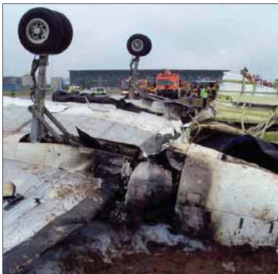
Photo No. 9: Left Engine Fire damage
