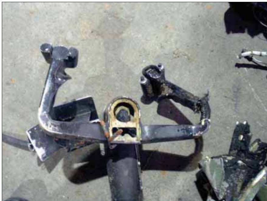
Photo No. 7: Co-pilot control wheel showing fracture of right-hand control grip
