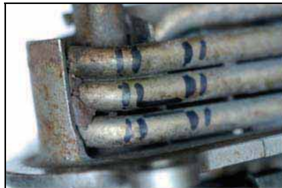
Photo No. 6: Possible sensing tube breach location
