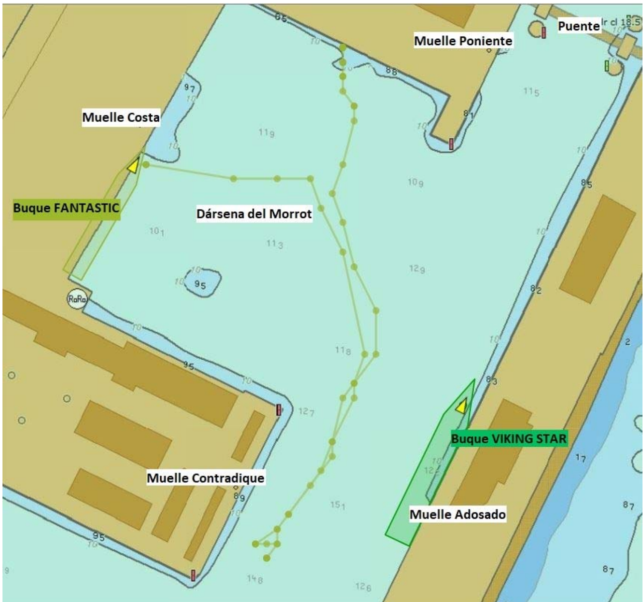
Figure 5. Maneuver performed by the FANTASTIC ro-pax vessel
