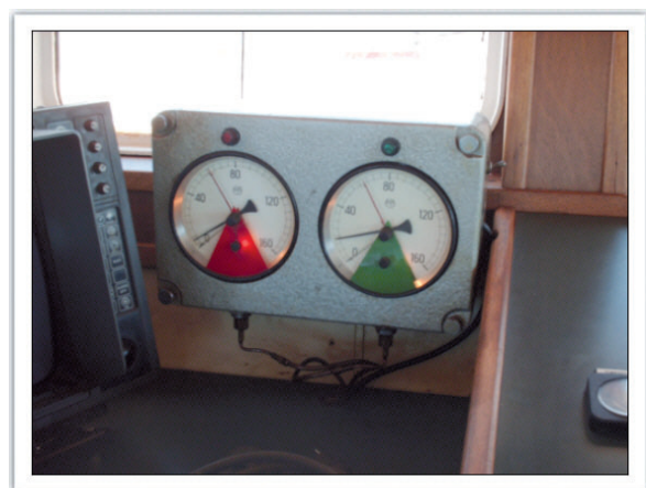
Figure 14. Tension indicators on the trawling machines, with adjustable alarm
