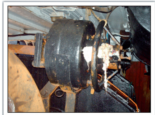
Figure 11. Trawling machine brake wheel with its actuator
