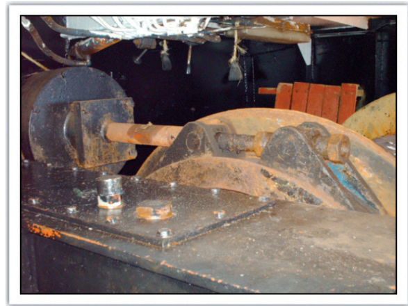
Figure 10. Trawling machine brake
