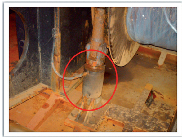
Figure 13. Trawling machine tension measurement force sensor
