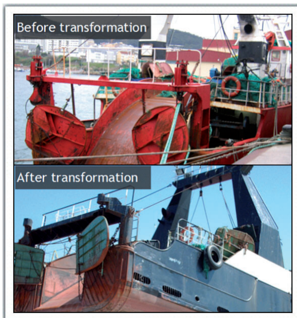
Figure 3. Modification of the gantry crane
