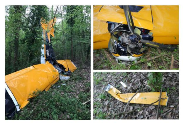
Figure 2. General view of aircraft (left). Close-up of engine and propeller (top right) and the detached slat fragment (bottom right)
